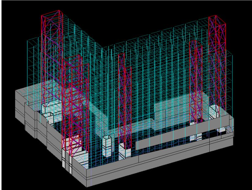
**Figure 5.3 – 3D Model with Braced Frames**
