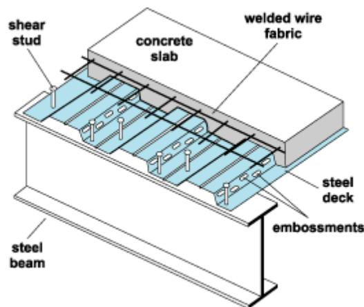
**Figure 3 - Composite Floor System with Metal Deck**
