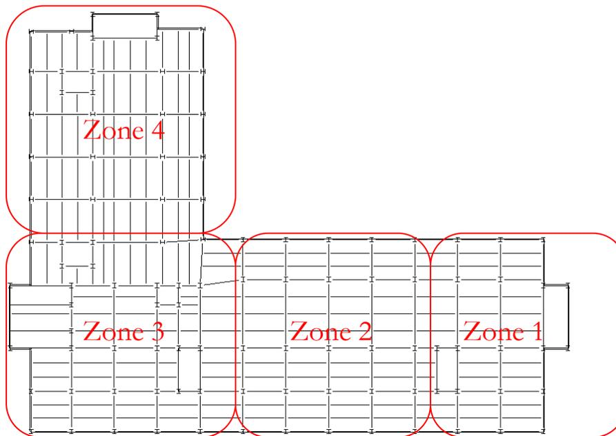
**Figure 7.2 - Concrete Framing Pour Zones**
