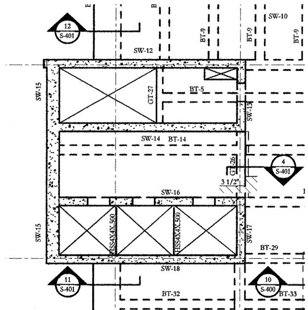
Figure 1.4 – Shear walls around Elevator Core
