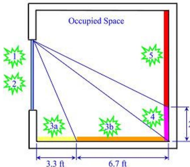
Figure 7.1 - Location of Glass during Explosion
