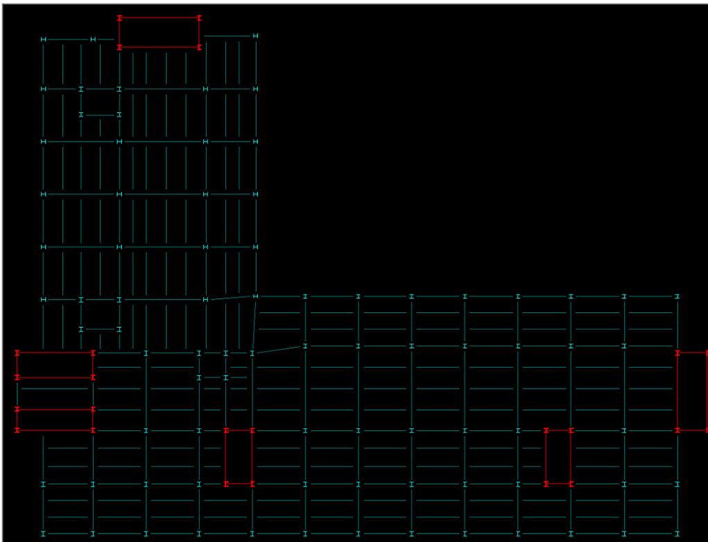
**Figure 5.4 - Plan View of Lateral Frames in Red**
