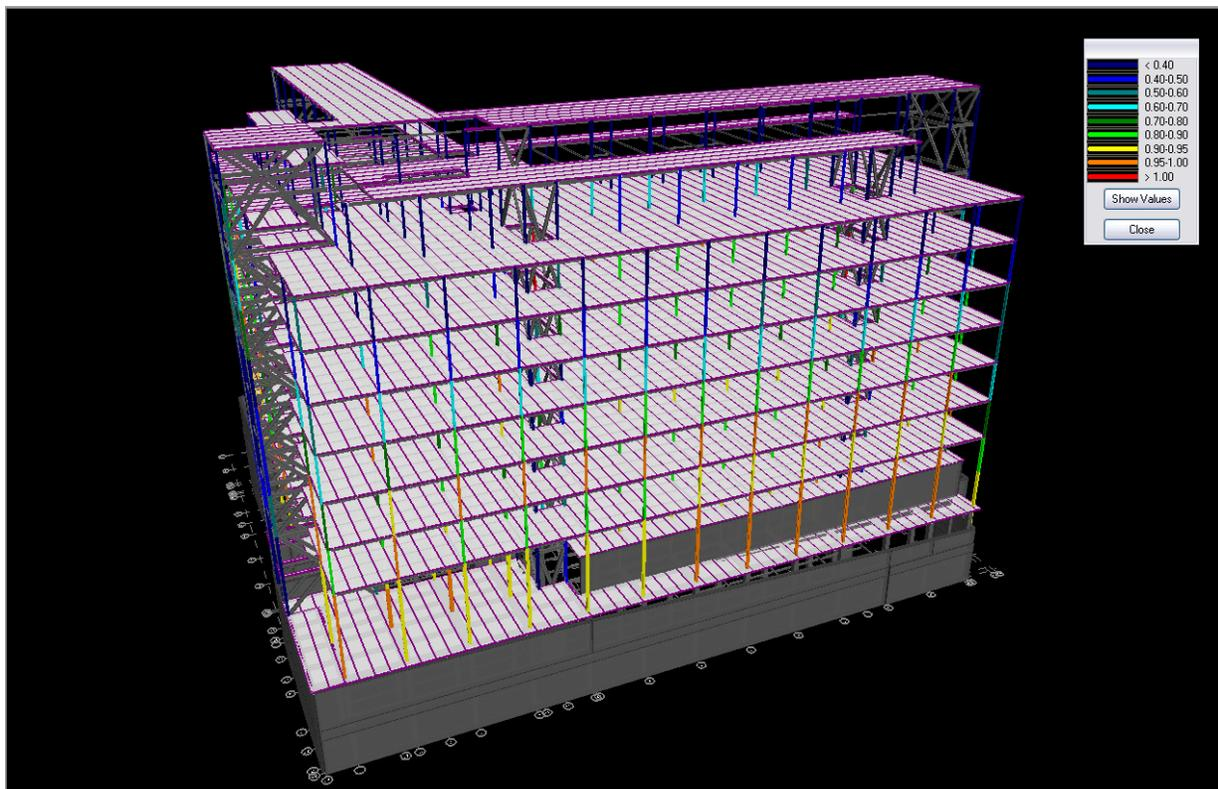
**Figure 5.2 - Column Layout with Code Check**
