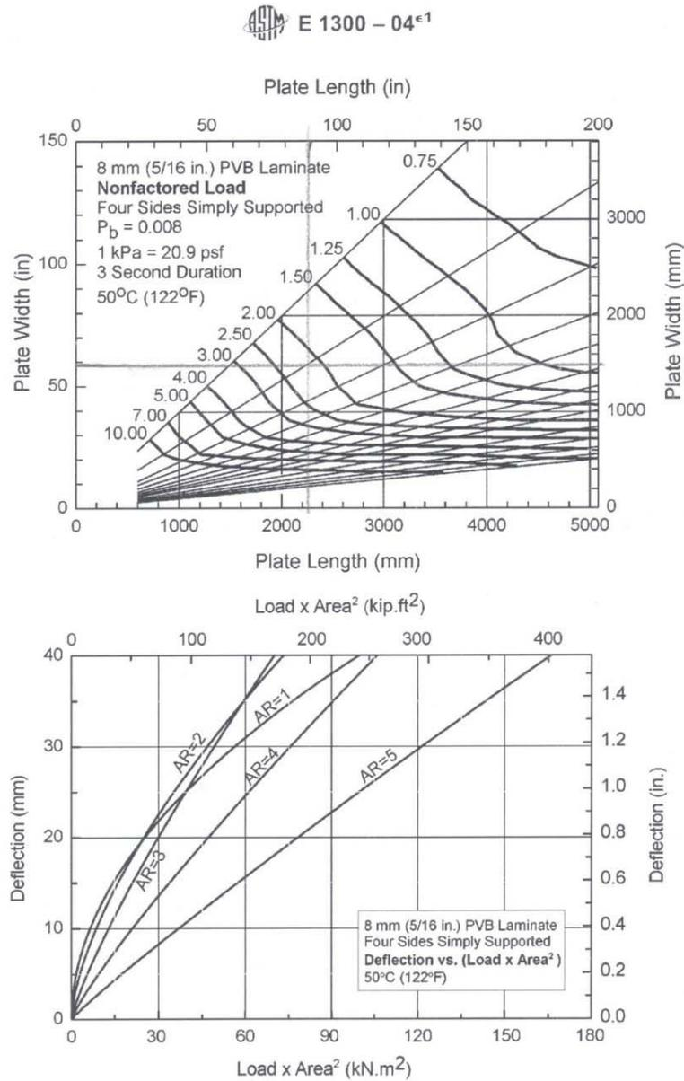
FIG. A1.29 (upper chart) Nonfactored Load Chart for 8.0 mm (5/16 in.) Laminated Glass with Four Sides Simply Supported
