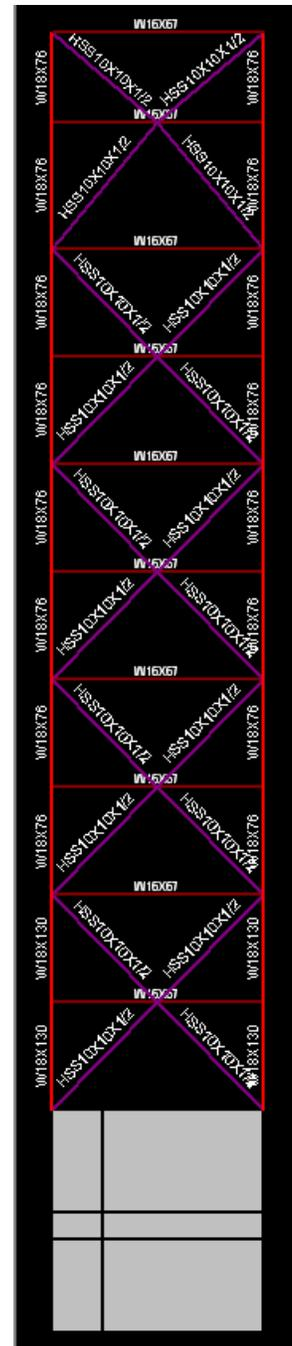
Figure 5.5 - Typical Modified "X" Braced Frame
