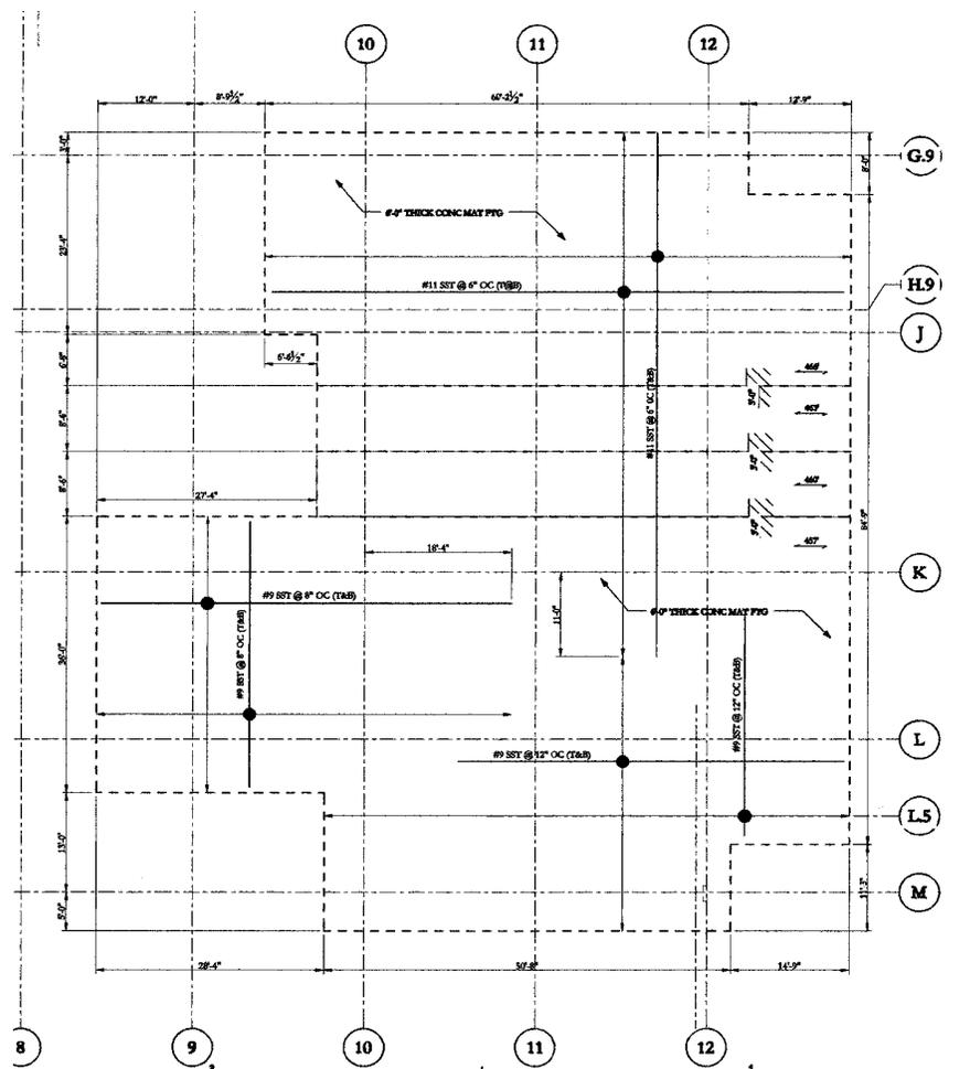
Figure 1.1 – Mat Foundation under Imaging Equipment
